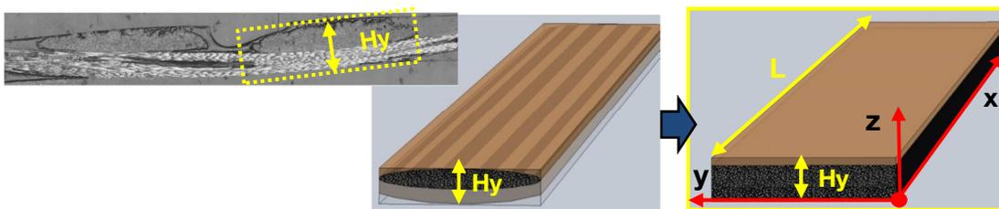
**Figure 1:** Characteristic tow morphology and rectangular tow equivalent used for modelling
