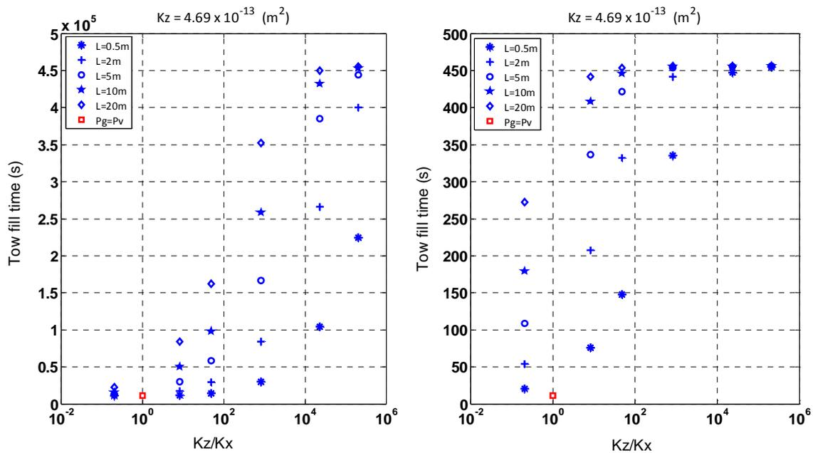
Figure 2: Time to fill a tow of various lengths and permeability ratios at 32°C – left and 130°C - right
